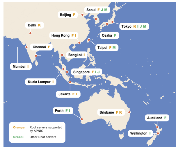
▲ Location and identity of root servers deployed in the Asia Pacific region.
